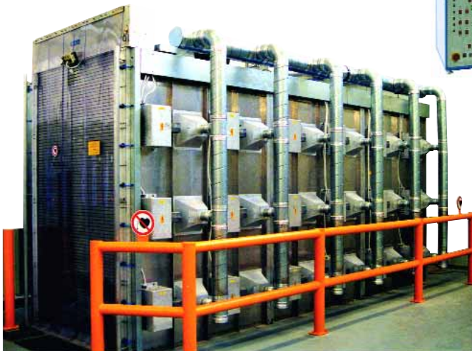
Mikrowellen-Kammertrockner Microwave chamber dryer 21 m 3 / 30 kW
