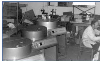
Induction casting units, 1970
